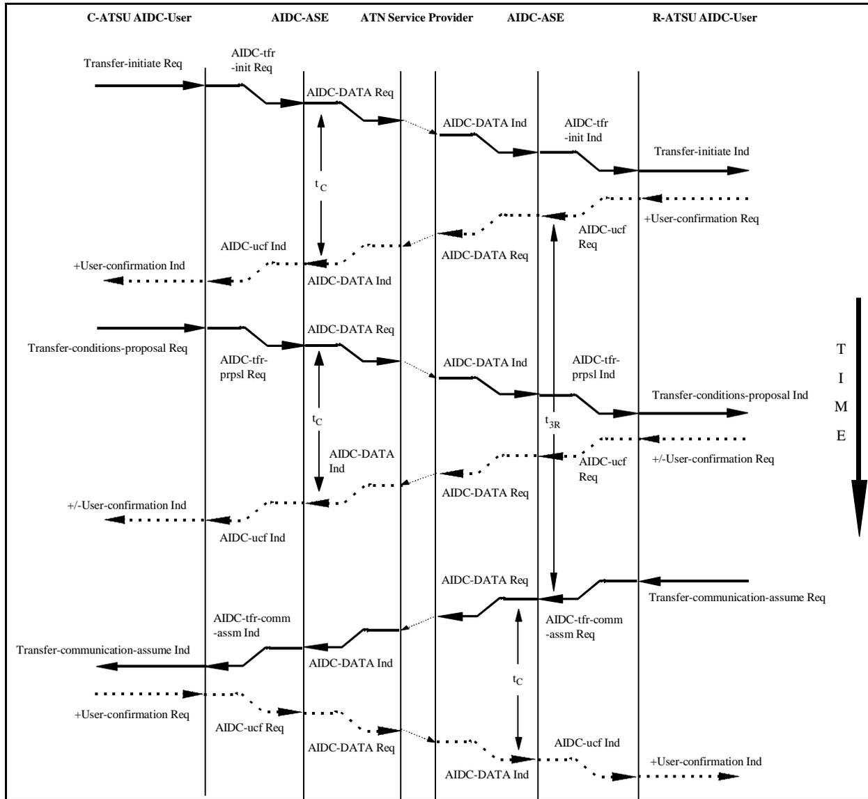
Figure 3.2.10-15: Sequence Diagram showing the invocation of the Transfer-conditions-proposal service, with the predicate P1 false, followed by the invocation of the Transfer-communication-assume service
