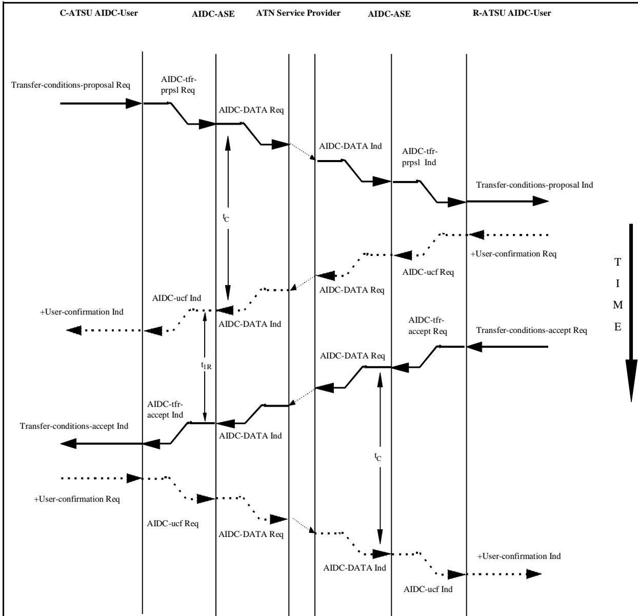
Figure 3.2.10-16: Sequence Diagram showing the invocation of the Transfer-conditions-proposal service and the Transfer-conditions-accept service with the predicate P1 true
