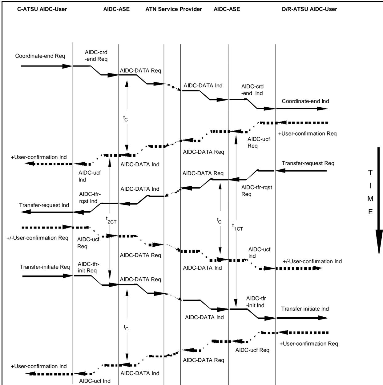
Figure 3.2.10-10: Sequence Diagram showing the invocation of the Transfer-request service
