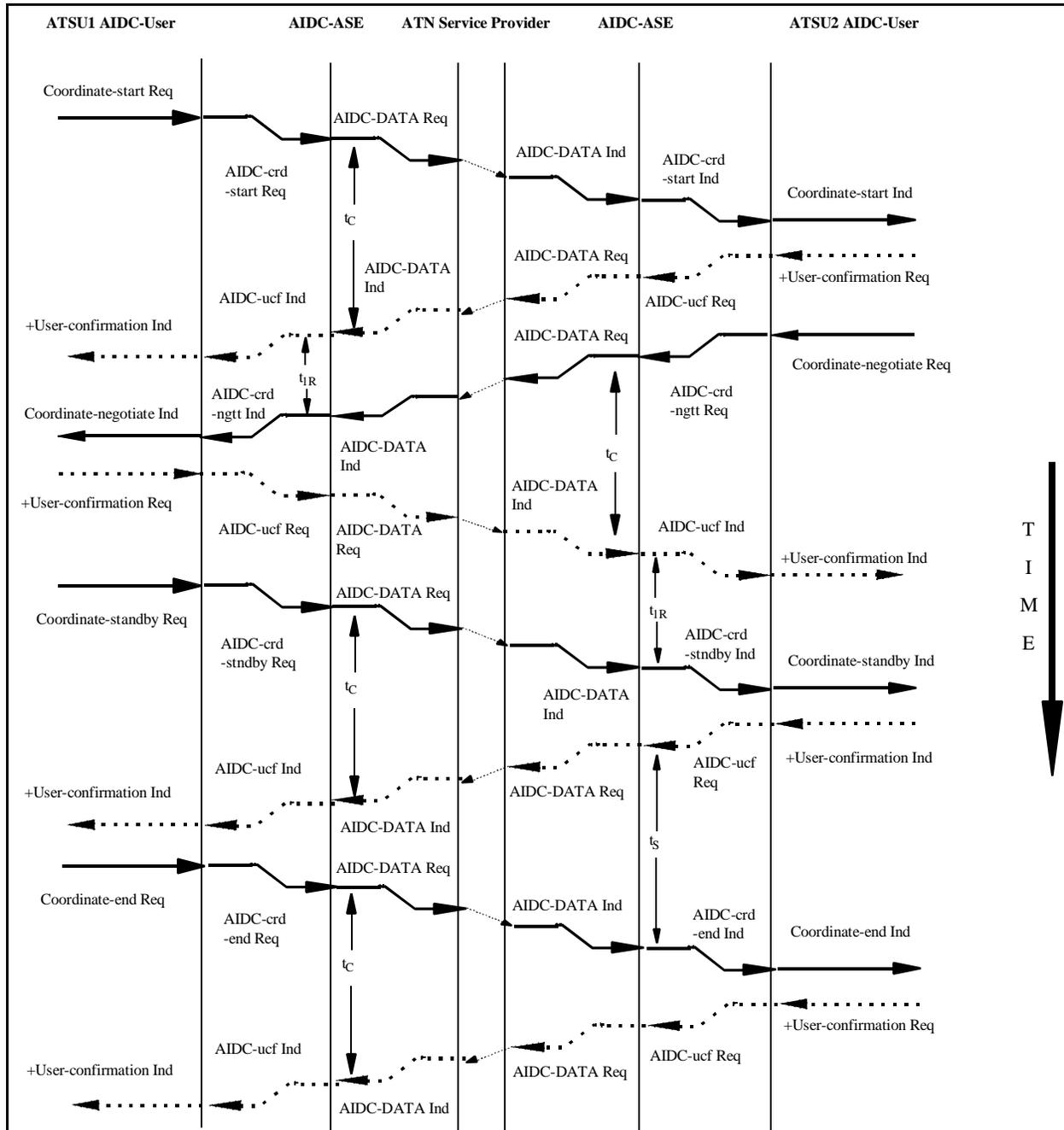
Figure 3.2.10-7: Sequence Diagram showing the invocation of the Coordinate-standby service followed by the Coordinate-negotiate service
