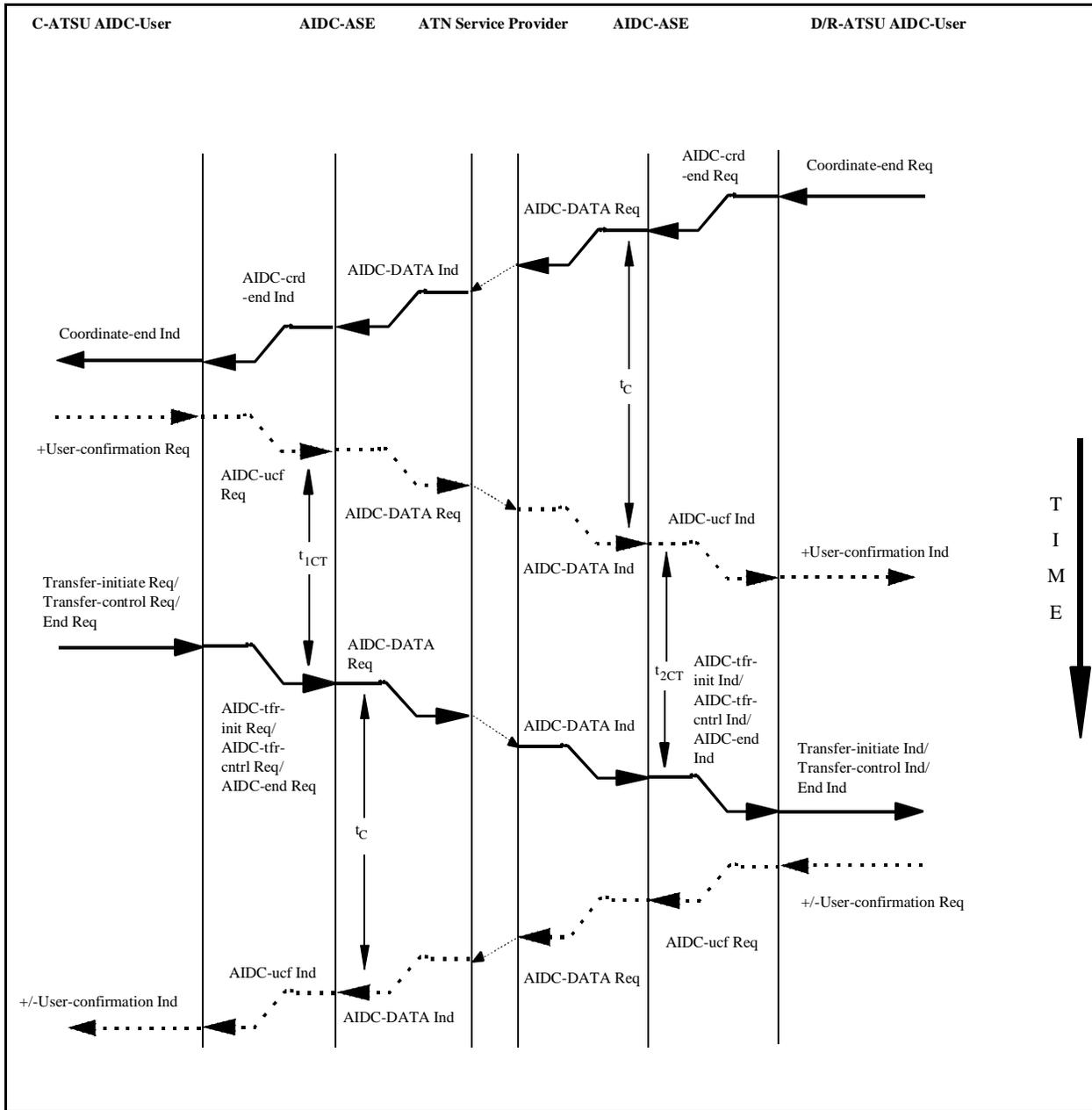
Figure 3.2.10-9: Sequence Diagram showing the start of the Transferring Regime through the invocation of the Transfer-initiate service
