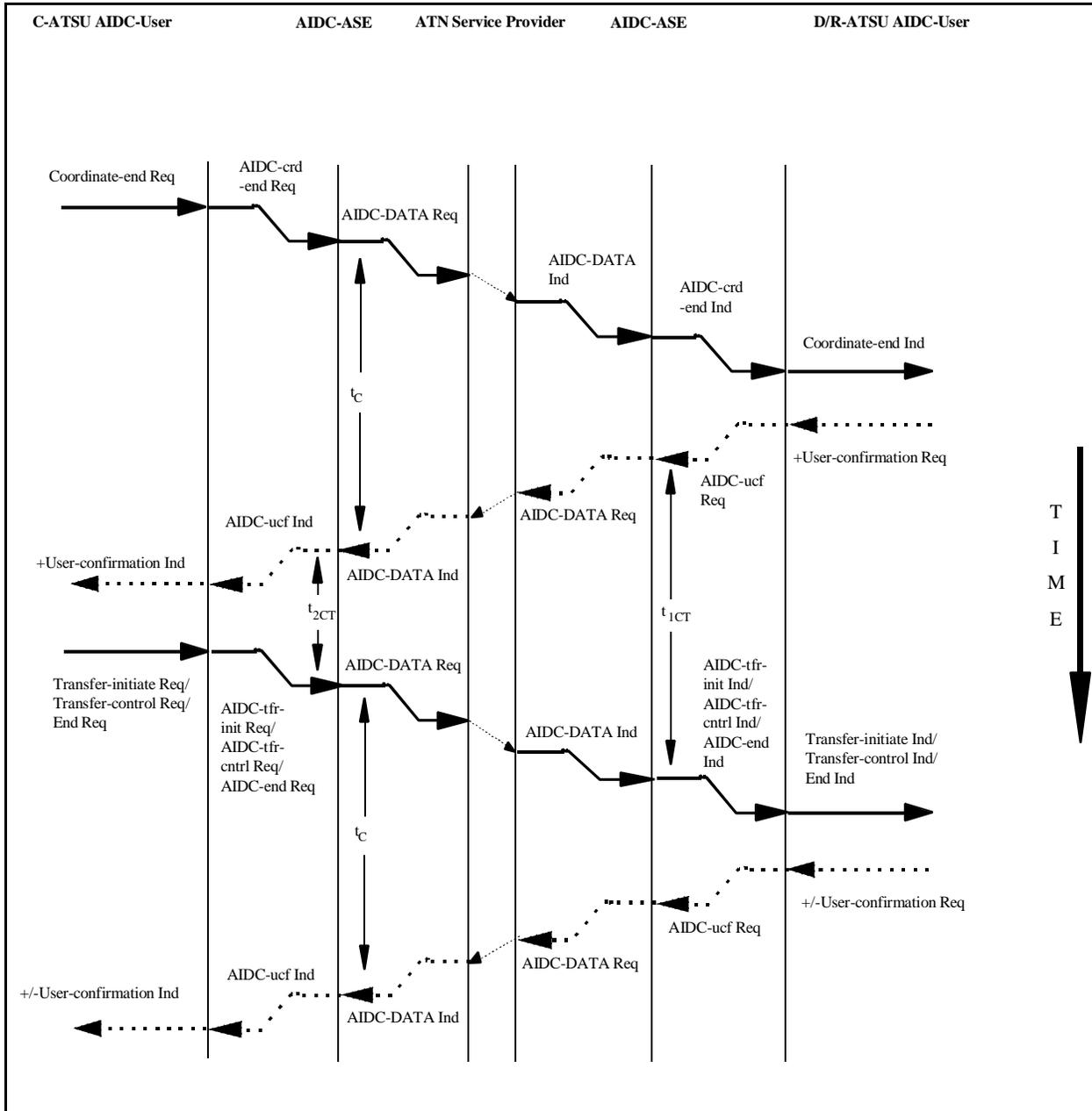
**Figure 3.2.10-8: Sequence Diagram showing the start of the Transferring Regime through the invocation of the Transfer-initiate service**
