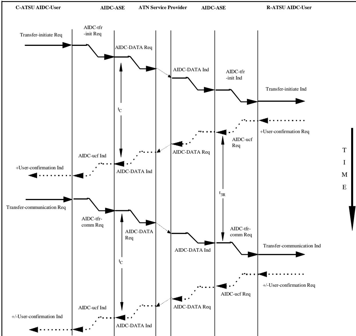
**Figure 3.2.10-12: Sequence Diagram showing the invocation of the Transfer-communication service after the Transfer-initiate service**
