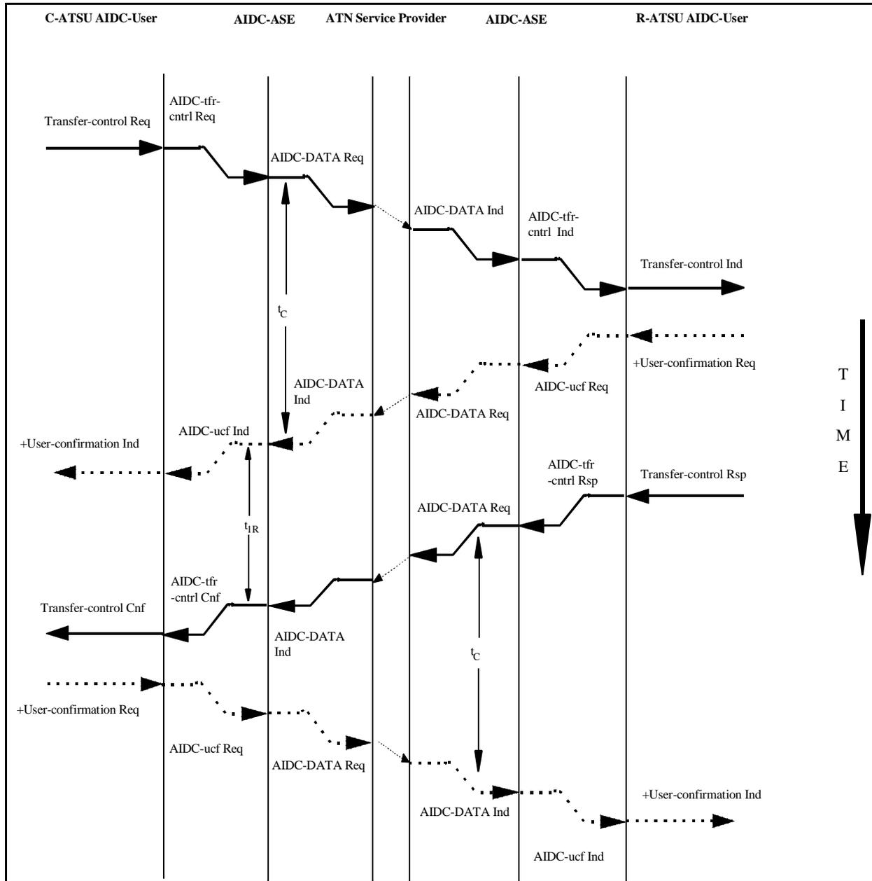
Figure 3.2.10-19: Sequence Diagram showing the start and end of the Transferring Regime through the invocation of the Transfer-control service
