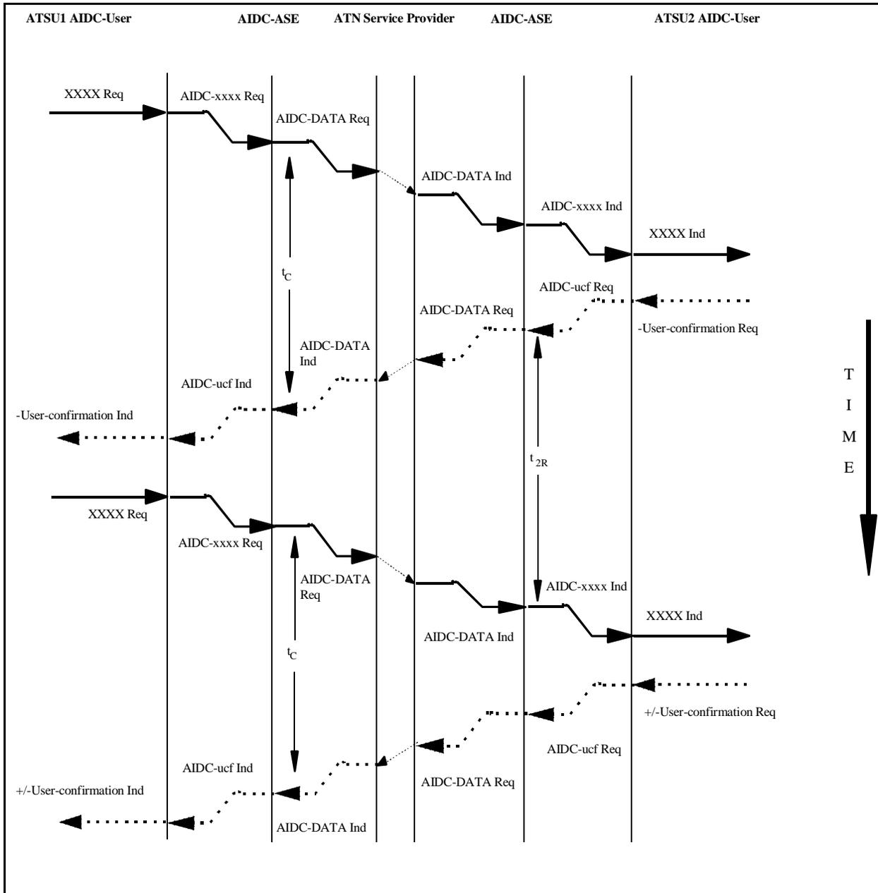
**Figure 3.2.10-25: Sequence Diagram showing the sequence for a negative User Confirmation for all services except the Transfer-request, Transfer-conditions-proposal, Transfer-conditions-accept, and Info-Transfer services**
