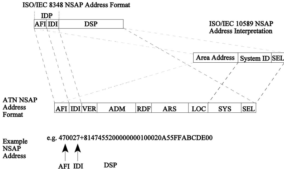
**Figure 5.4-3 Derivation of the ATN NSAP Address Format**
