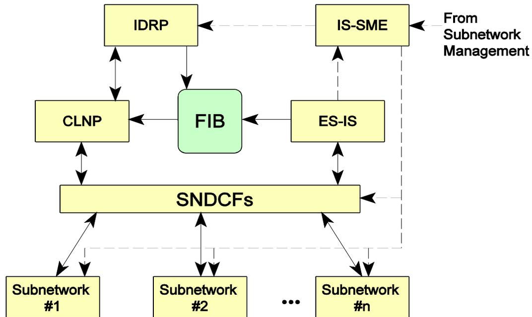
**Figure 5.3-1 Assumed ATN Router Architecture for Air/Ground Route Initiation**
