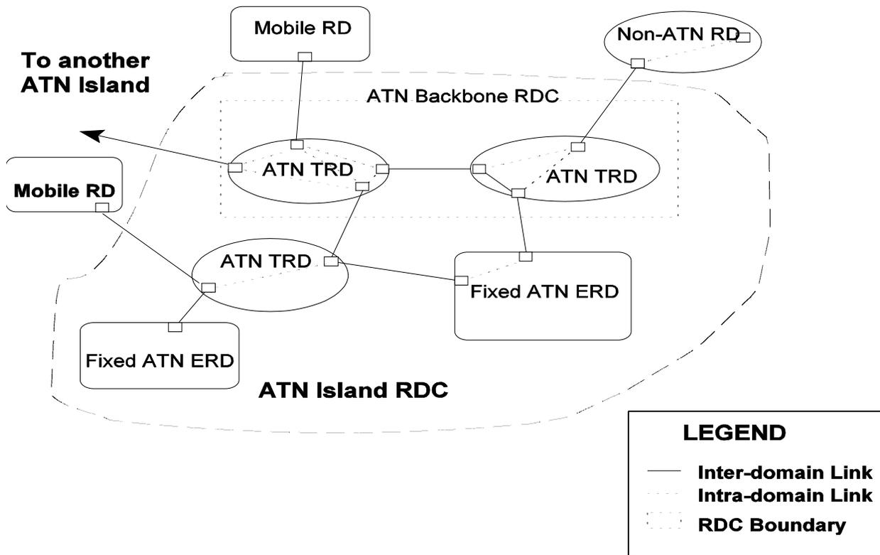
Figure 5.2-1 Example ATN Island Routing Domain Confederation Structure
