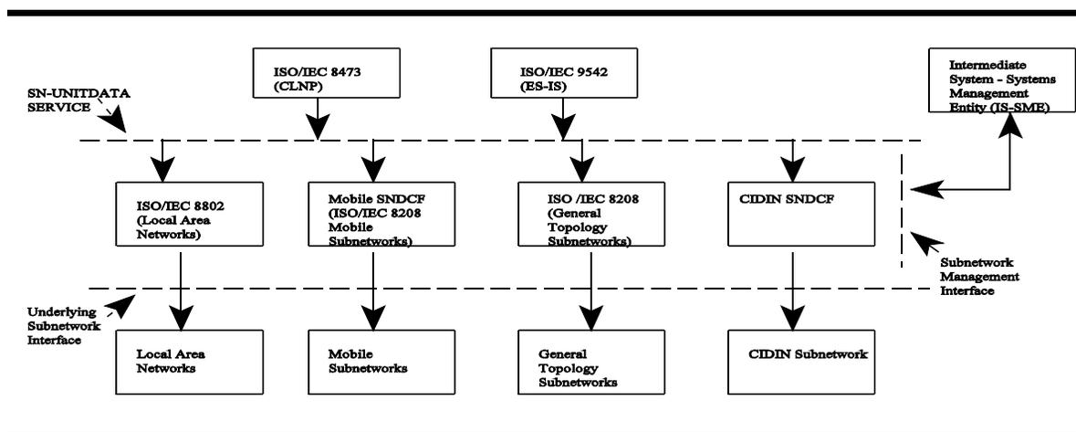
Figure 5.7-1 Relationship of SND CFs to SN-Service and underlying Subnetworks
